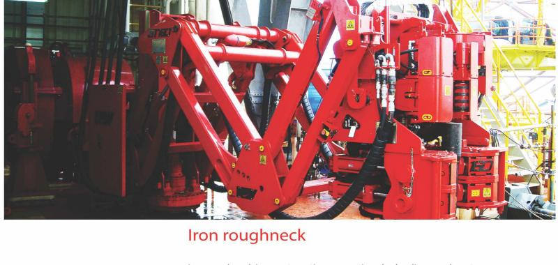
Iron roughneck is an automatic pneumatic or hydraulic wrench system that serves as breakout and make up tongs to make or break tubular on the drilling rig floor.
